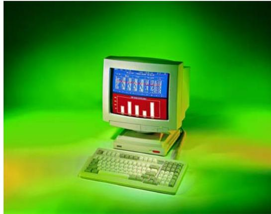
The ADD5 4000/260 LFC (color) and ADD5 400/260 LF (monochrome) text terminals provide a compact logic unit for use with any VGA display. They are an ideal solution for customers looking to use Wyse display terminals in legacy applications. A full emulation set includes Wyse 50/50+, WY-60, the DEC VT-100, VT-220, VT 320, TeleVideo 925, ADD5 Viewpoint, PCTerm and SCO Console. The 4000/260 LFC (color) also supports Wyse 350 and WY 325.
